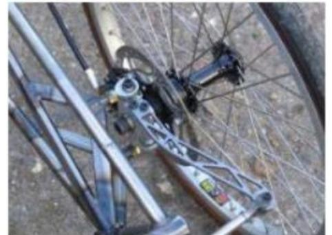
In respect of the wheels, the forks give more support than the hub, but the hub saves weight. Wheels that will take side load are essential. BMX wheels for example, **not Plastic**.
